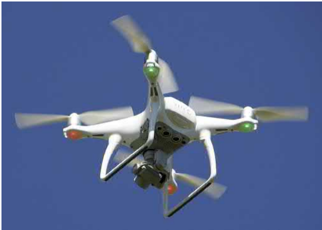
Fig. 1-9 Small UAV, DJI Phantom, a quadcopter that has become quite popular. Note the red and green signal lights that aid the pilot in flying the drone. Flown by D. Van der Merwe.
